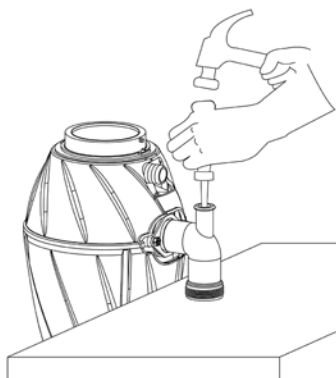
Removal of the diaphragm
